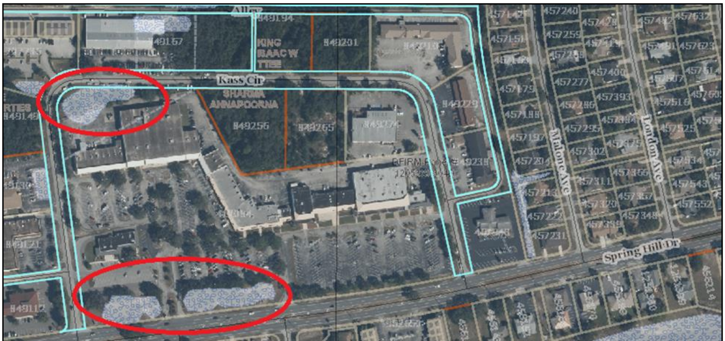
Figure 26: Drainage Retention Areas (DRAs) in Front of Spring Hill Drive and Behind Spring Hill Plaza
