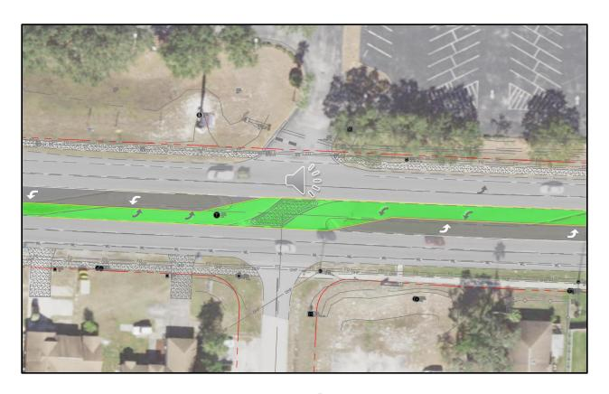
**Existing:** directional median opening -> **Proposed:** closed median opening
