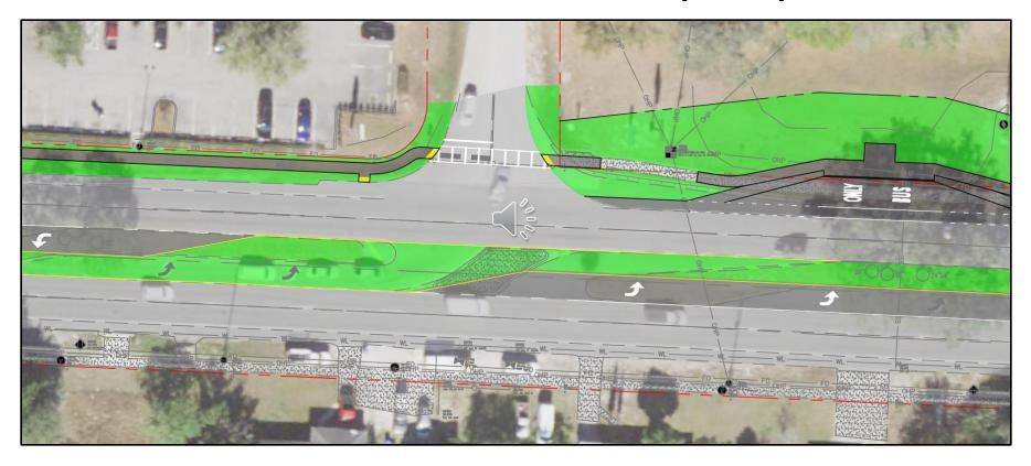
**Existing:** directional median opening  $\rightarrow$  **Proposed:** closed median opening
