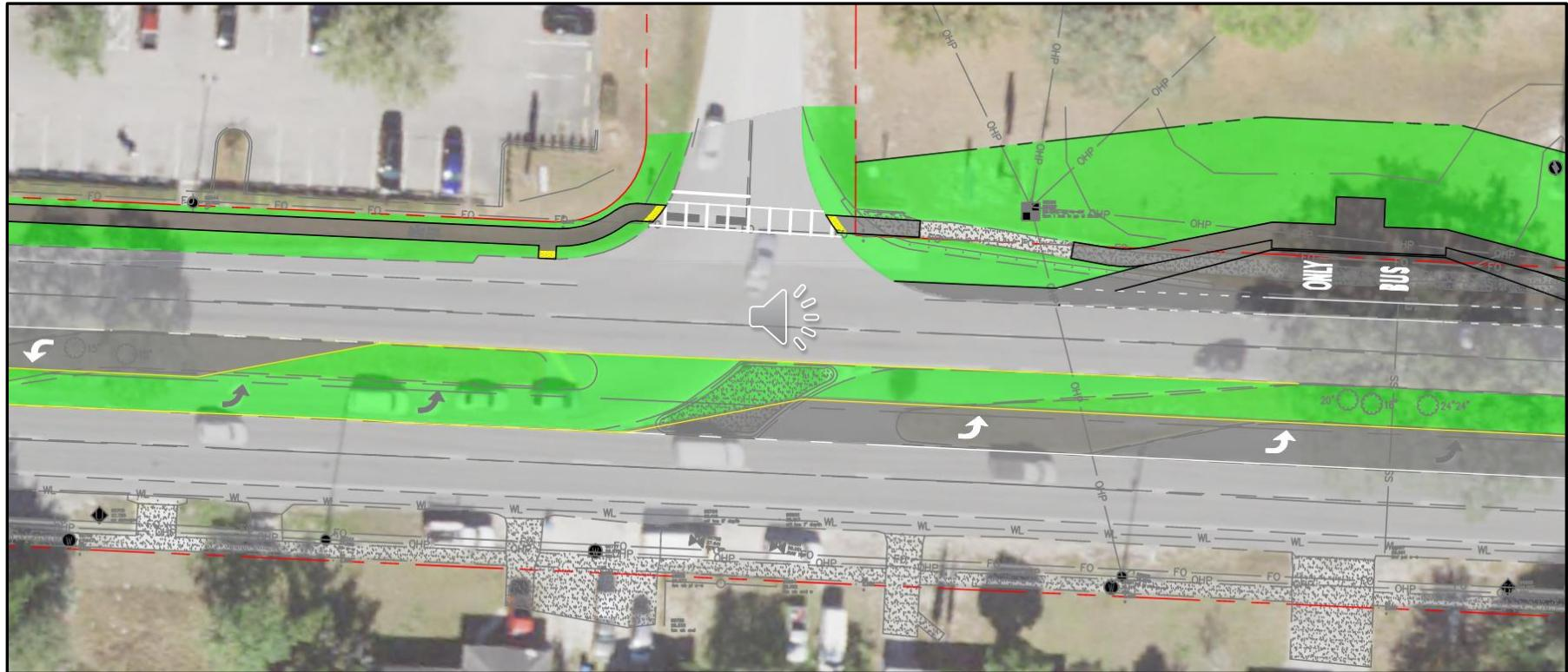
Existing: directional median opening → Proposed: closed median opening
